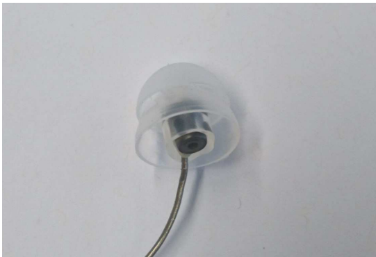
Figure 2: Sennheiser KE3 microphone in a silicone dome.
