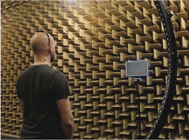
Figure 4: The feedback system consisting of a head tracker on the subject's head and a monitor outside the critical radius, giving feedback on the head movement.
